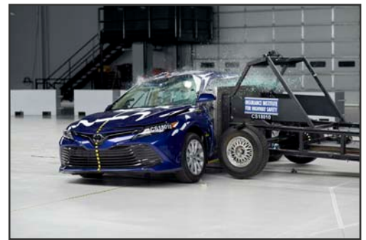
Test vehicle is struck by a movable barrier in a side impact research crash test
