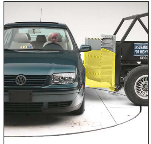
NHTSA barrier, shown in yellow, superimposed over taller IIHS barrier
