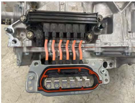
Figure 1: Cables between transmission motor windings and inverter.
