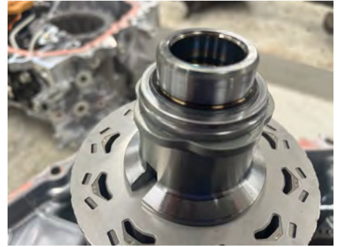
Figure 3: Resolver Trigger Mechanism
