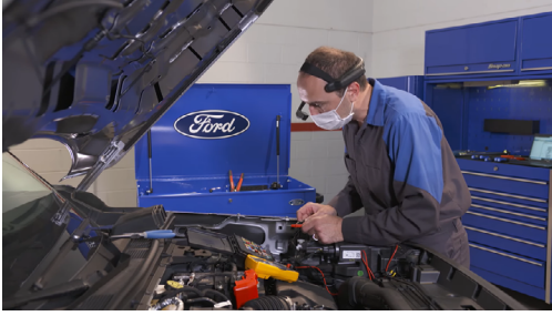
The two-way, hands-free electronic headset, known as See What I See (SWIS), allows for both visual and audio communication between the dealership technicians and team members at the Technical Assistance Center.
