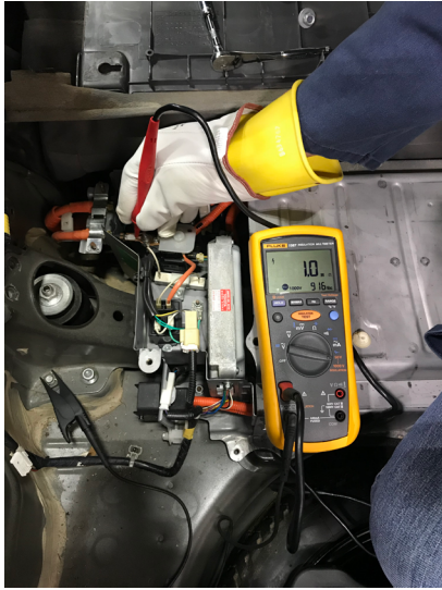
Figure 1: Use of isolation meter.
